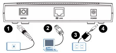
1 GEPON: Connect an SC-type, single-mode optical cable to this port for Internet access.
